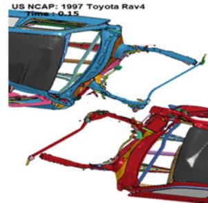
Fig. 7 The simulated collision process between two SUVs collides with a 40% deviation at a speed of 55 km/h
