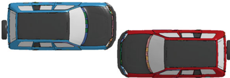
Fig. 6 Simulation of a collision between two SUVs with a 40% deviation
