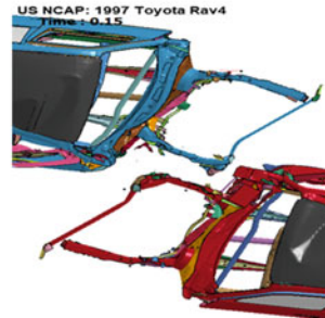
Fig. 7 The simulated collision process between two SUVs collides with a 40% deviation at a speed of 55 km/h
