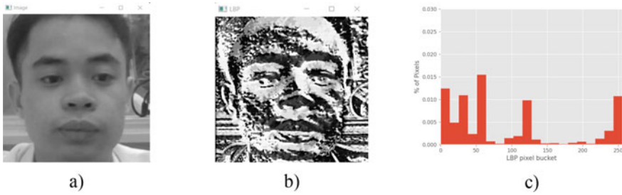
Fig. 2 a The pre-training image; b The LBP training image; c The LBP pixel bucket of the sample image
