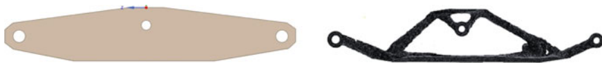
Fig. 2 Original structure and its shape after topology optimization of the input link
