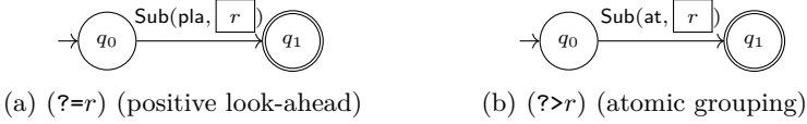
Fig. 3: a conversion from (la, at)-regexes to (la, at)-NFAs. For negative look-ahead, we use the corresponding kind label nla. For positive and negative look-behind, besides using the kind labels plb and nlb, we suitably reverse \boxed{r} .
