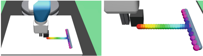
Fig. 3. Visualization of the generated curriculum goals in the FetchPush task. The colors (ranging from red to light blue) represent the curriculum goals across different episodes of the training. The gray color represents the desired positions. (Color figure online)
