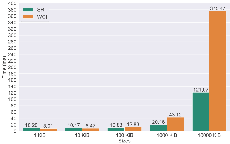
Fig. 4. Comparison of average processing times for a minimal HTML page with inline (WCI) or linked (SRI) JavaScript of different sizes
