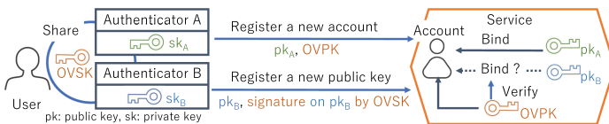
Fig. 1. Registering Public Keys Using An OVK
