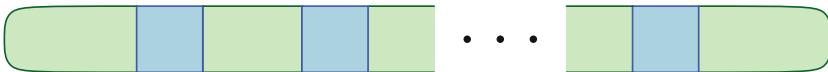
Fig. 5. Each tunnel consists of two end tunnel segments and various middle tunnel segments, separated by crossing boxes.
