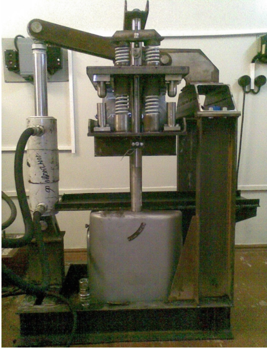
Fig. 5. General view of the press with electric vibration drive
