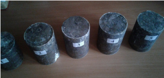
Fig. 6. Polymer concrete samples for presented structural composition [14]
