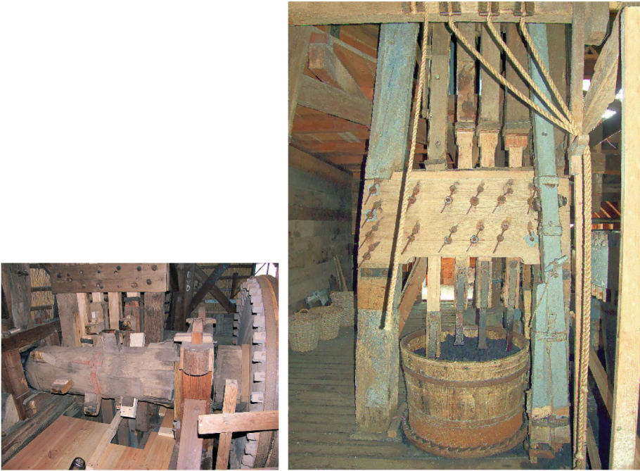
Fig. 18. Cam axis of the chopper and the chopper in the paper mill De Schoolmeester (Source: Wikipedia).
