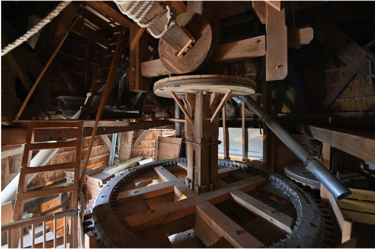
Fig. 25. Sack hoist in the Laren mill.
