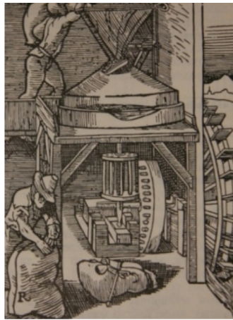
Fig. 2. Vitruvius hydraulic flower mill. (Source: forum/go.php ).
