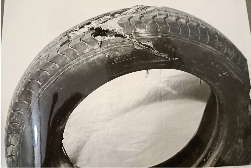
Fig. 3. Picture number 24 included in the committee’s report: the burst tire
