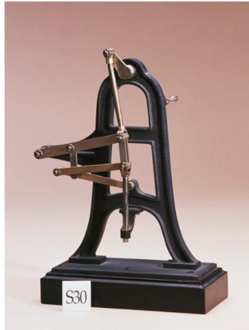
Fig. 4. Six Link, Straight-Line Mechanism of Chebyshev [12]
