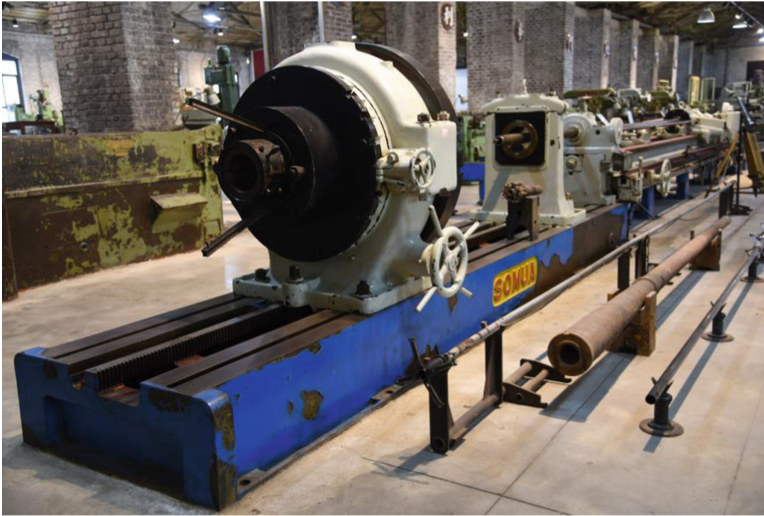
Fig. 9. SOMUA Rifling Machine for Rifling the Barrel of the 36 Type Mountain Gun (Photo by LIU Guihong)
