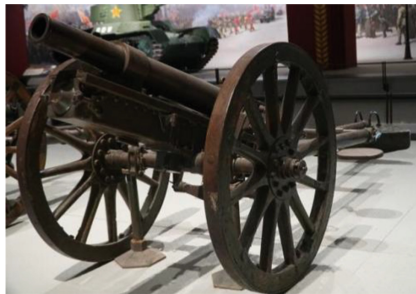
Fig. 3. The picture on the right shows a Jin-made 13 Type 75 mm Mountain Gun in the Chinese People's Revolutionary Military Museum (Photo by the author).
