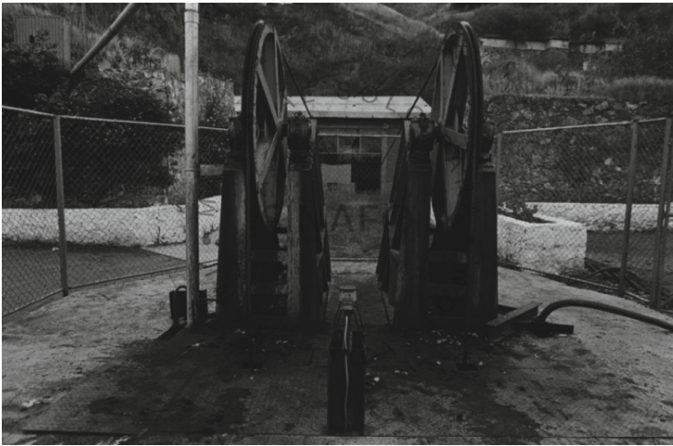
Fig. 8. Lifting pulley with steel cables ( http://mediateca.inah.gob.mx/repositorio/islandora/object/fotografia%3A485386 )
