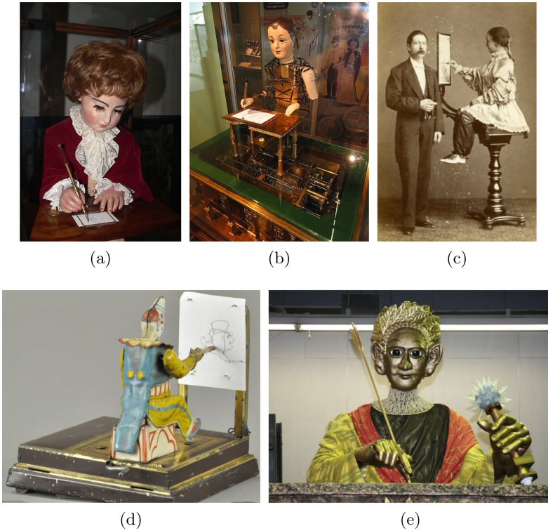
Fig. 1. Drawing automata: (a) the draughtsman by Jaquet-Droz; (b) Maillardet's automaton; (c) John Nevil Maskelyne's Zoe automaton; (d) the mechanical artist by Phillip Vielmetter; (e) replica of Gakutensoku by Makoto Nishimura.
