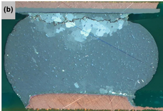
Fig. 1. Crack in the solder ball due to thermal loading.[15]
