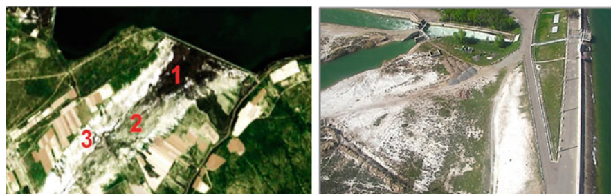
Fig. 7 Soil salinization downstream of dams. On the left – the Karazhantak dam, Sentinel-2 image (1 – bog solonchak soils, 2 – highly saline meadow soils, 3 – solonchaks. On the right – solonchaks in downstream and on the lower slope of the dam [14]
