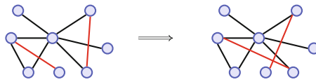
(b) Adding noise by swapping nodes in two randomly selected edges. Left: Original network. Right: Network after one edge swap.
