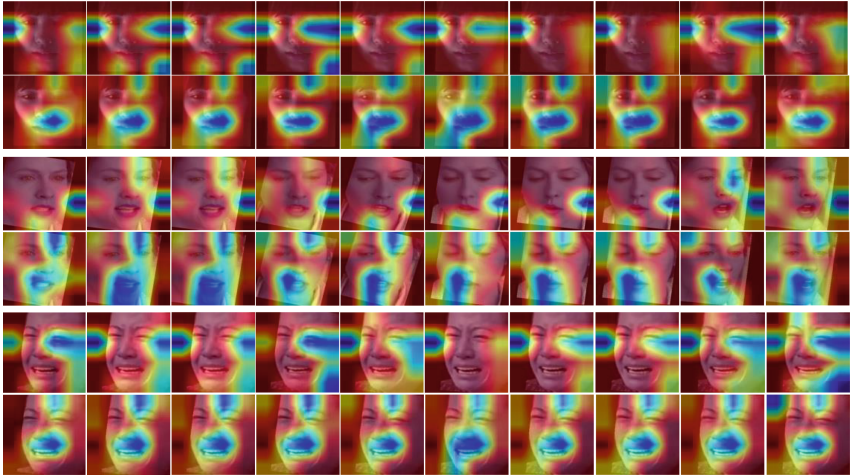
Fig. 3. Visualization of the learned feature maps. There are three sequences are presented, which including the facial expression of Neutral, Anger and Sadness, respectively. For each sequence, the images in the first row are heat-maps generated by the Former-DFER, and the images in the second row are heat-maps generated by DSGCN.
