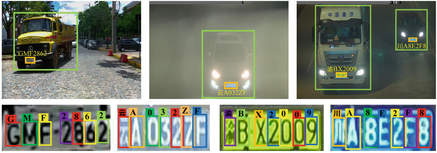
Fig. 5. Visualization examples of license plate detection and recognition.
