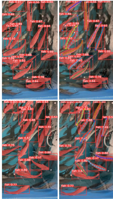
Fig. 1. Yolov8l based detection & pixel-length estimation using splines on our dataset.
