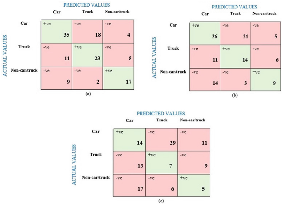
Fig. 18. Confusion Matrix using AdaBoost algorithm: (a) Haar-like; (b) HOG and (c) LBP.
