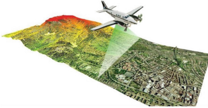
Fig. 3. Example of airborne LiDAR scanning method [35]
