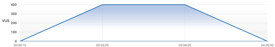
Fig. 11. Soak testing - VUs progress over time
