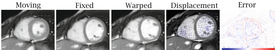
Fig. 2. Evaluation of the registration results. This results were achieved by our proposed method. The error represents the difference between the warped and fixed images.
