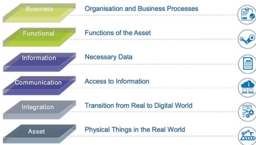
Fig. 6 RAMI 4.0 Functional Architecture (Schweichhart, 2016)
