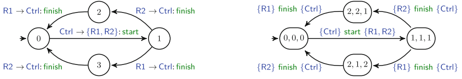
Fig. 4. Choreographic Automaton (left), extended with multiple senders and receivers, and composed TA (right) of the automata in Fig. 1
