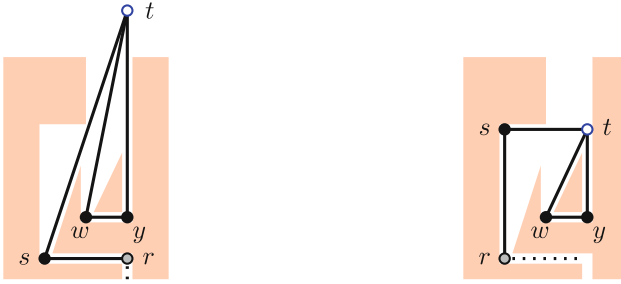
(a) State false where vertex t is above the forbidden area of the gadget. This is also the base situation appearing in \Gamma and \Gamma' . (b) State true where vertex t is inside the cavity formed by the forbidden area of the gadget. This state can only be reached if the split or crossing gadget below has orientation top.
