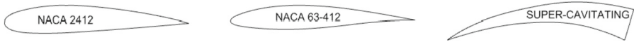
Fig. 4. Three different types of profiles: NACA 2412 (left), which is widely used to many aeronautical applications for low Re numbers; NACA 63–412 and Super-Cavitating (centre and right, respectively), two examples of profiles used to design hydrofoils.
