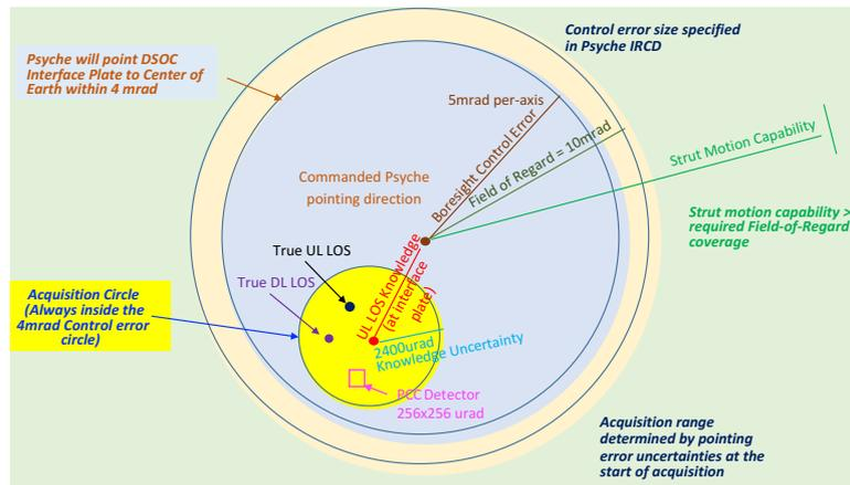
**Figure 4. Pointing Uncertainties Associated with Initial Uplink Beacon Acquisition**
