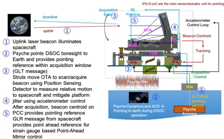
**Figure 1. System Architecture of DSOC Flight Laser Transceiver with Key Components**
