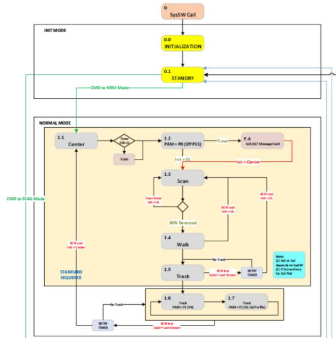
Figure 2. Operational Sequence Diagram of DSOC FLT
