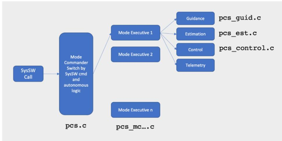
**Figure 8. PCS Software Execution Diagram**
