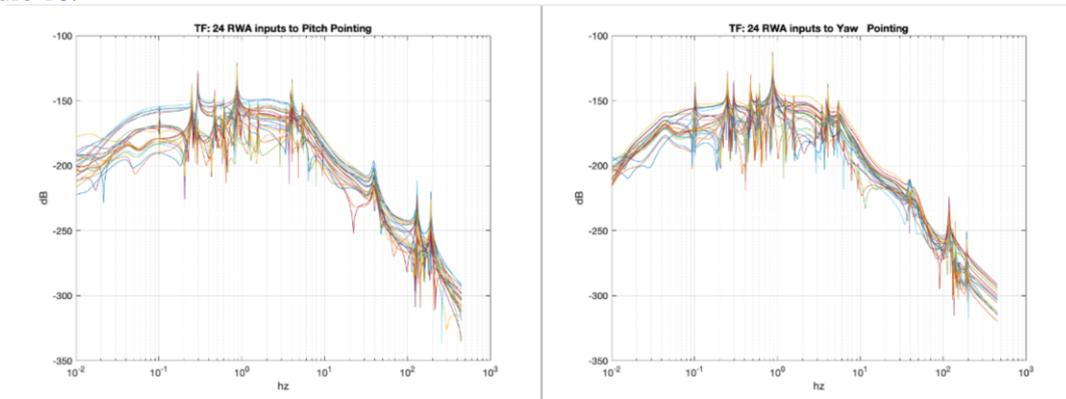
**Figure 16. Transfer Functions from RWA Force/Torque to LOS Pointing**
