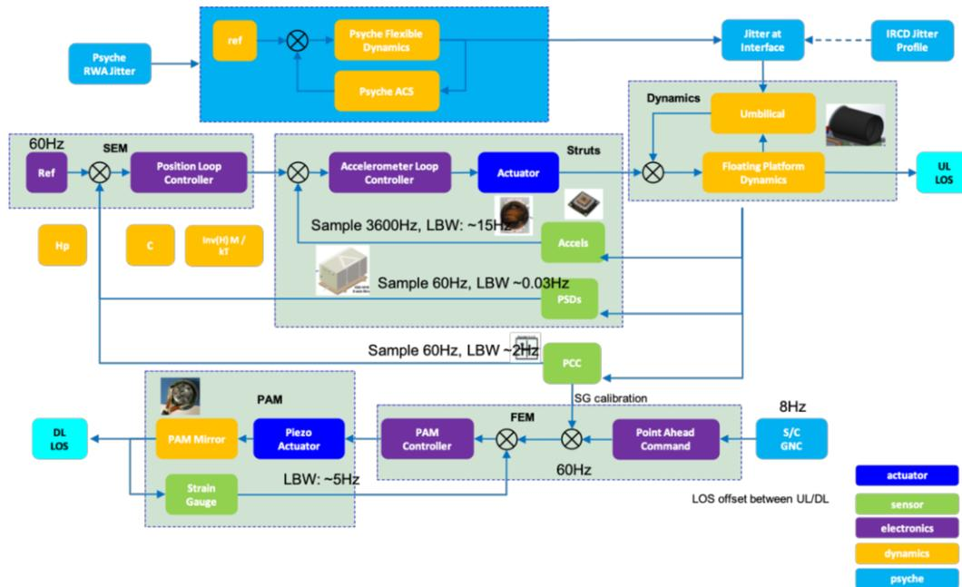
Figure 10. DSOC Platform Control and Downlink LOS Control Diagram
