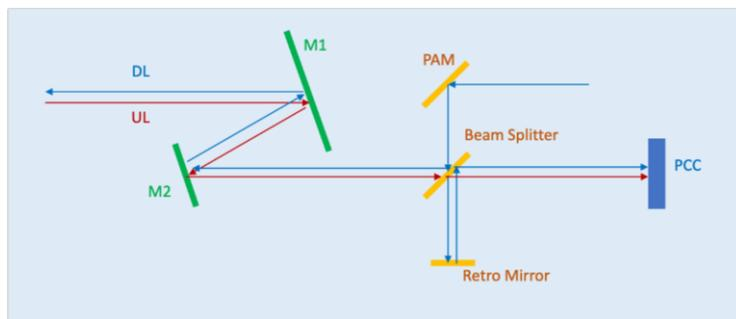
**Figure 5. Flight Terminal Optical Transceiver Assembly**
