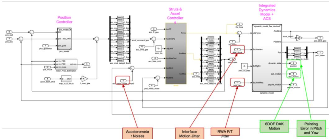
**Figure 15. Frequency Domain Sensitivity Analysis Model**
