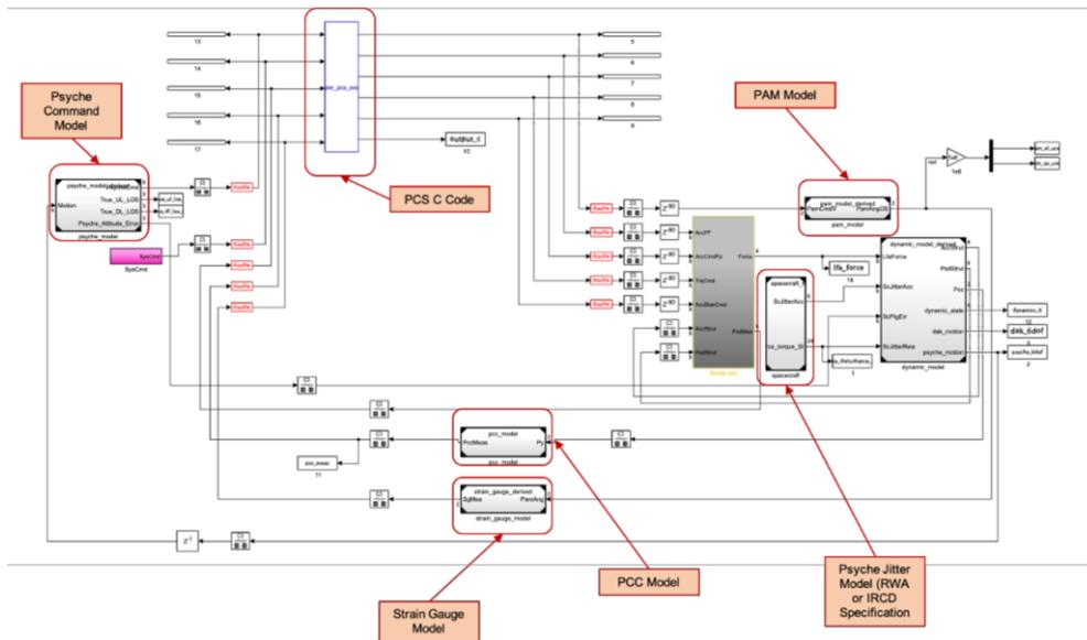
Figure 17. Time Domain Performance Simulation Model
