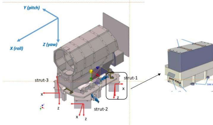
**Figure 6. Isolation and Pointing Strut (IPA-S) and Their Placement on DSOC FLT**
