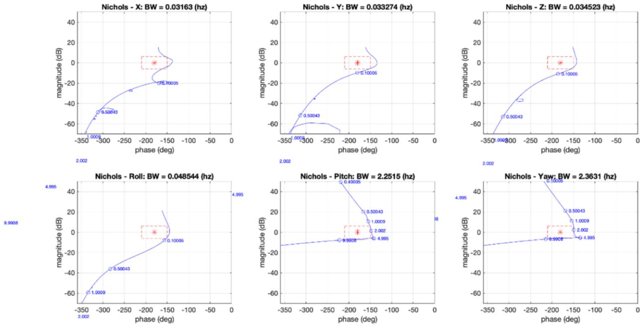
Figure 14. SISO Position Loop Stability Results
