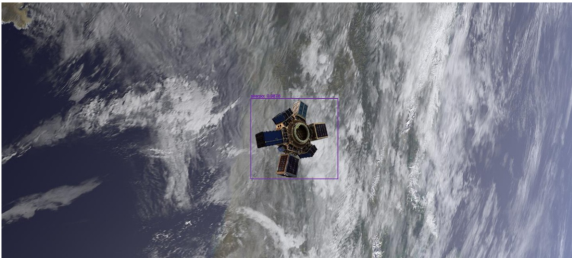
Figure 12. Synthetically-generated Spaceflight Sherpa OTV identified and located in a space environment at range, emulating sensors and algorithms flying on Tanker-001.
