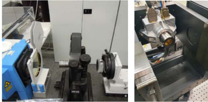
Figure 7. OH BB Interferometer test (left); OH BB mounted on performance test bench (right)
