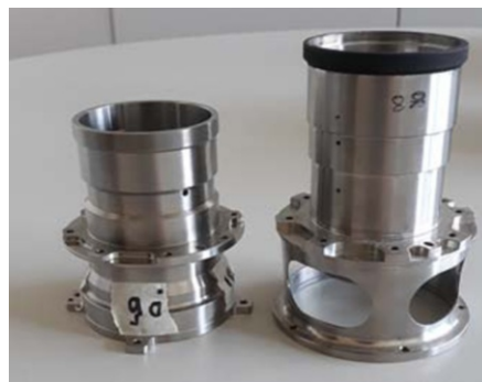
Figure 2. AA-STR MKII Optical Barrel (on the left) vs AA-STR Optical Barrel (on the right)
