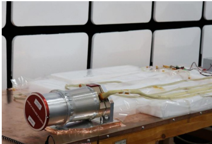
Figure 13. Photograph of the EMI test setup of the CT-2020.
