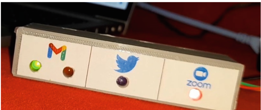
Fig. 12. Red LED switches on when a user is in a meeting
