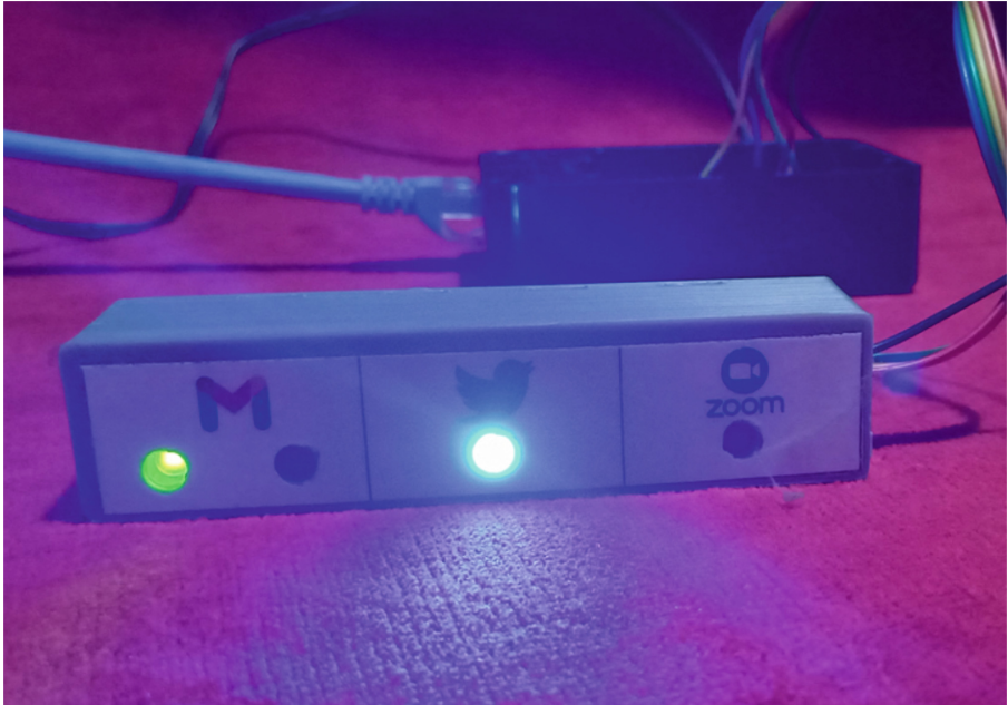
Fig. 11. Blue LED switches on when a user receives tweet alerts
