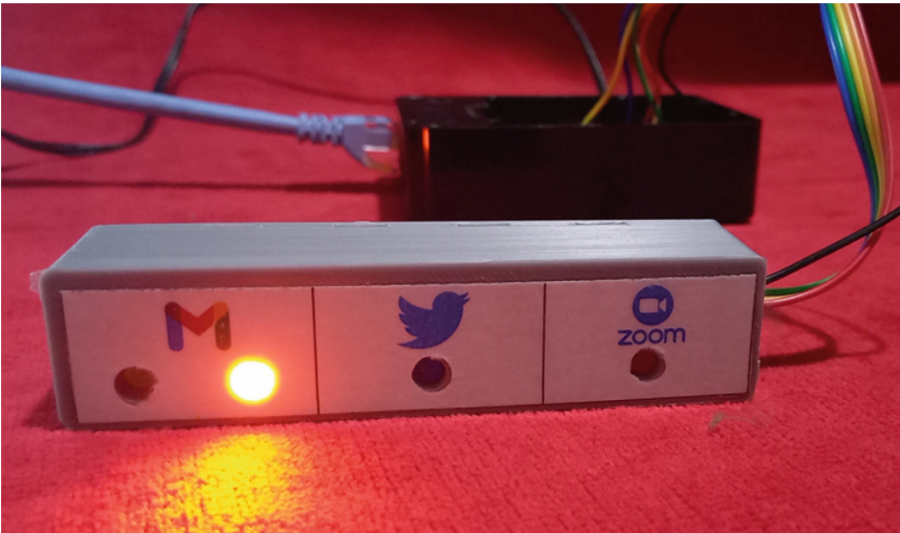
Fig. 10. Orange LED switches on when there are unread emails
