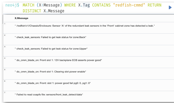
Fig. 8. A sample Neo4j cypher query to return those syslog messages which have been generated by the redfish-cmmd service.
