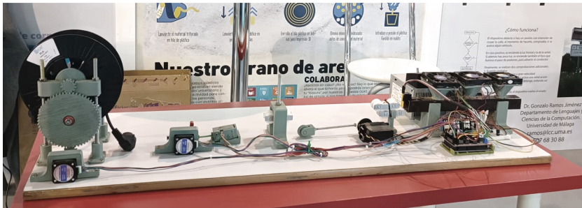
Fig. 8. Recycled plastic filament winder exposed at Foro Transfiere 2023.
