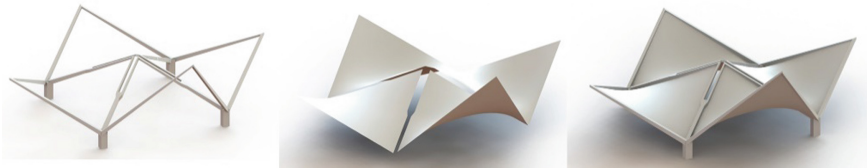
Fig. 8. The 4 Hyperbolic Paraboloids. Own elaboration.
