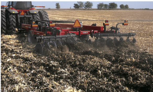
Fig. 2. Reduce tillage application (superficial is processed and the stubble remains on the soil surface)
