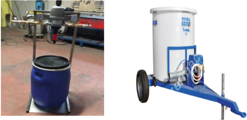
Fig. 1. Images of fertigation systems designed for hose reel irrigation machines.
