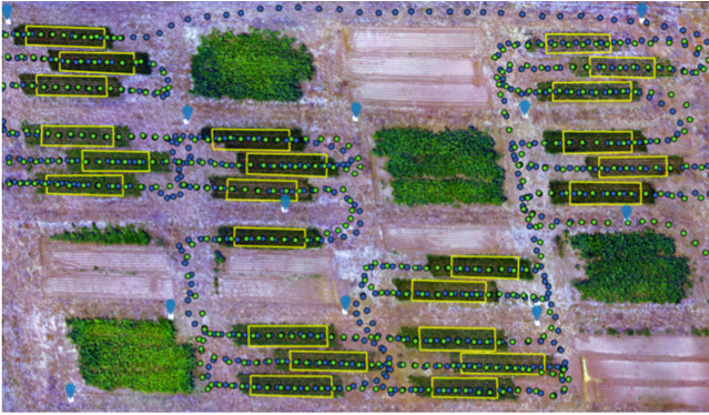
Fig. 5. RGB photo with ground control points (GCPs), data points, and plot boundaries overlaid in ArcGIS Pro 2.8 (blue teardrops show GCP's, yellow boundaries show reduced plot boundaries, green points show pre-harvest data points, and blue points show post-harvest data points).
