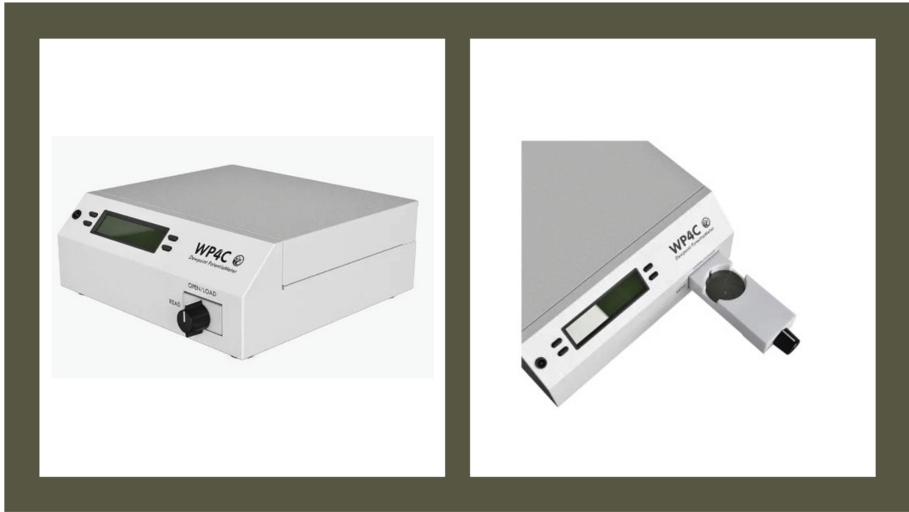
Fig. 1. Image of the WP4C on left shows the front side view with headspace closed. On right is the WP4C with headspace open showing location of sample cup.
