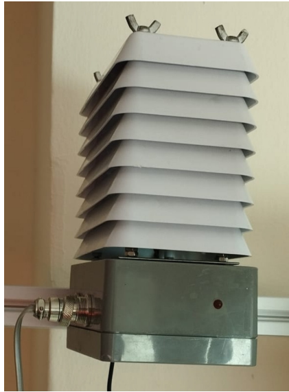
Fig. 2. Sensor shield and electronic control box
