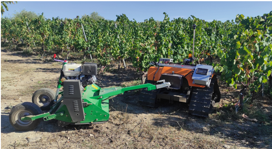
Fig. 1. The electric autonomous ground vehicle (AGV) coupled with a self-propelled mower during weed control trials in vineyards.
