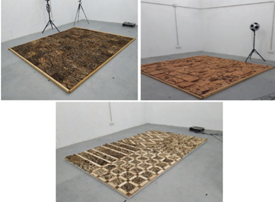
Fig. 3.3 Cork-based acoustic panels with different designs [29]
