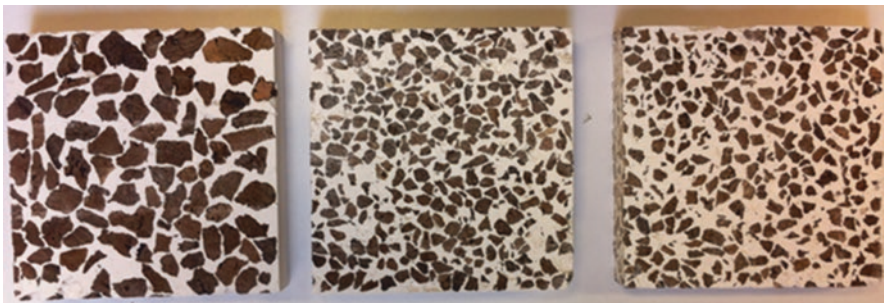
Fig. 2.1 Macroviews from gypsum-based composite materials including cork granules [11]
