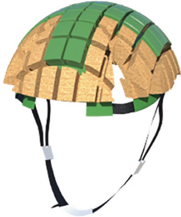
Fig. 5.4 Flattie – a new helmet concept designed specifically to improve the safety of e-micromobility users [36]
