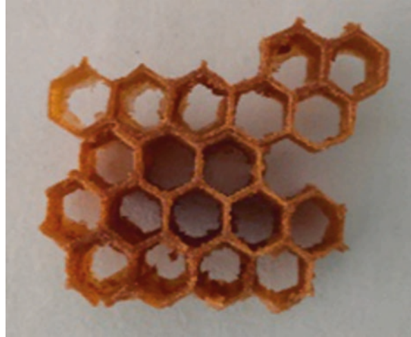
Fig. 2.2 Additively manufactured honeycomb structure made from photo-curable resin and cork powder [13]
