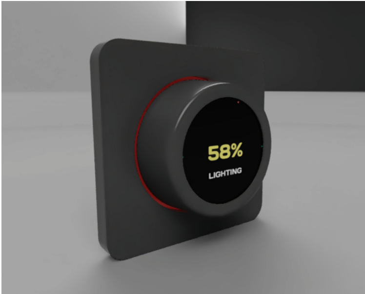
Fig. 5. Controller housing design
