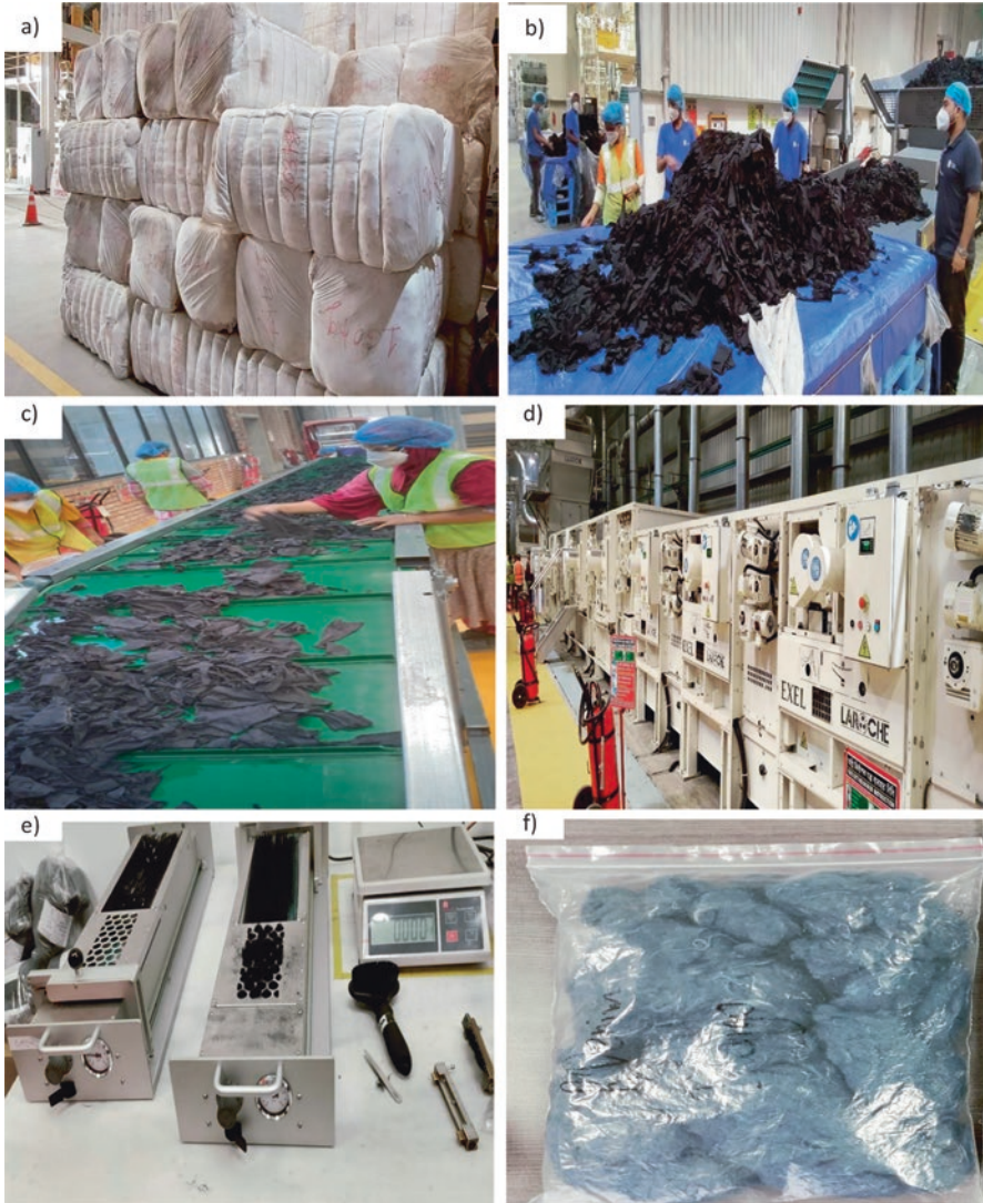
Fig. 4 Different sections of the mechanical fiber recycling industry: (a) collection of waste from available sources, (b) manual sorting and putting the pieces into the conveyor belt for cutting, (c) manual checking of the size of cut pieces for the required length after cutting, (d) main shredding operation to open fibres from fabric cut piece, (e) checking quality parameters of shredded fibers and (f) ready fiber for spinning. (Author generated)
