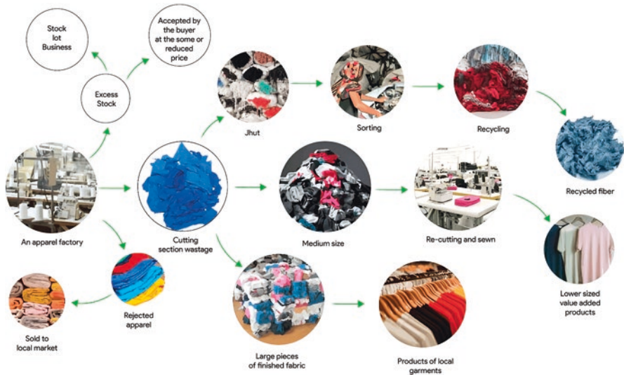
Fig. 3 Traceability of post-industrial textile and apparel waste in Bangladesh (Khairul Akter et al., 2022)
