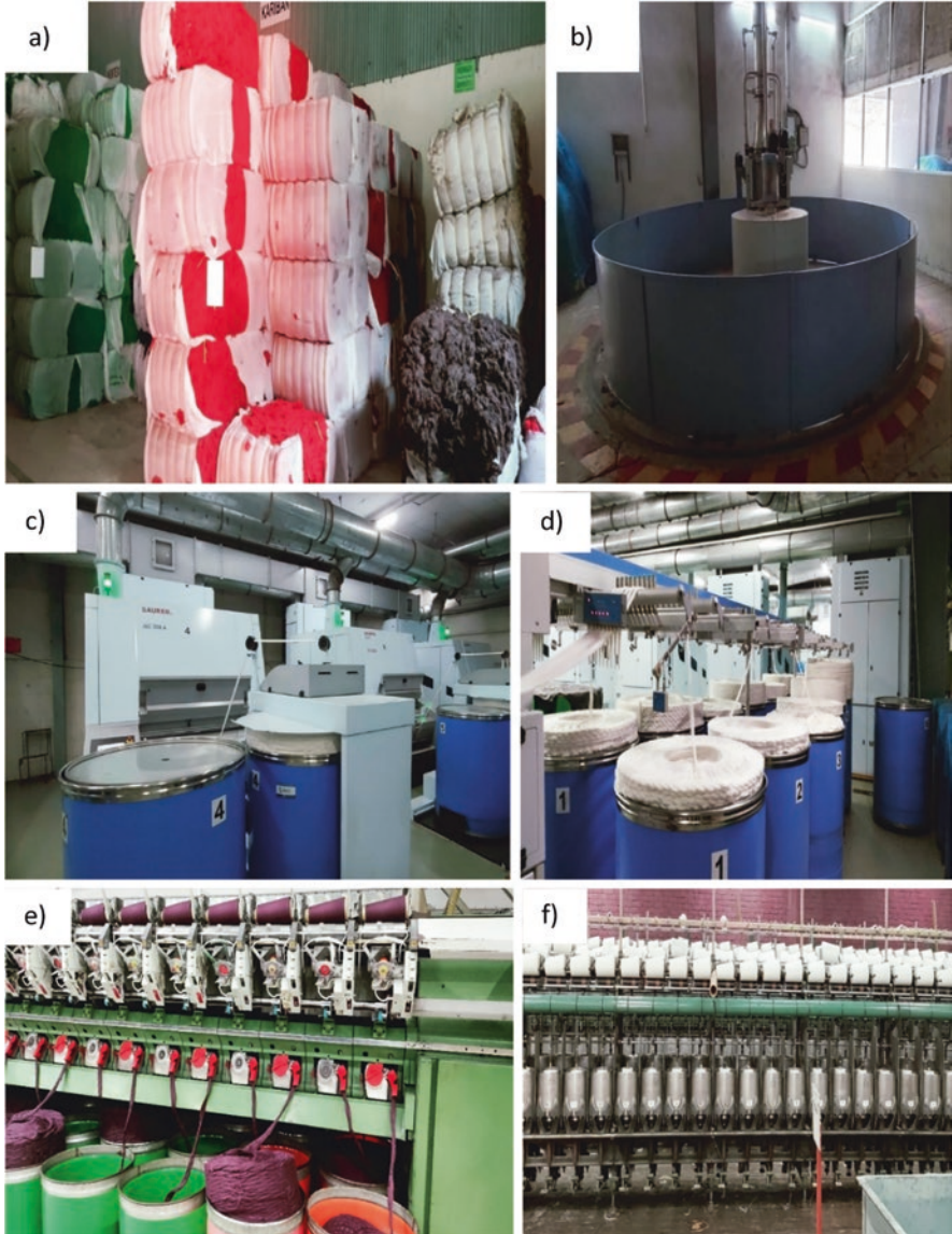
Fig. 6 Different sections of rotor spinning industry: (a) collection of recycled polyester and organic cotton fiber for mixing, (b) Blendomat, (c) carding machine for rotor spinning to handle short fibers, (d) carded slivers, (e) rotor spinning machine, and (f) doubling and twisting of sweater yarn. (Author generated)
