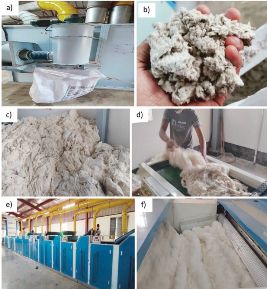
Fig. 5 Fiber recovery process from a different section of the spinning industry: (a) collection of waste from blowroom and carding process, (b) carding “Noil,” (c) collection of leftover and rejected slivers and yarn, (d) feeding the spinning waste into the shredding machine, (e) shredding machine for spinning waste (i.e., noil, rejected slivers and yarns), and (f) recycled fibers after the shredding of spinning waste. (Author generated)
