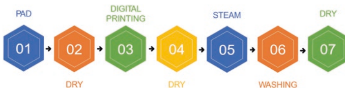
Fig. 6 Process sequence for digital printing
