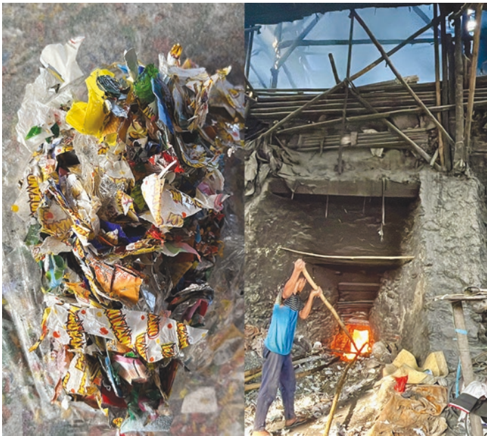
Fig. 10 (Left) Dried shredded plastic waste from paper mill company prepared to be used as fuel in a tofu factory. (Photo credit: Yuyun Ismawati). (Right) Discarded plastic waste from paper companies, sponges, and tires used as fuel to burn lime in Karawang. (Photo credit: Yuyun Ismawati)
