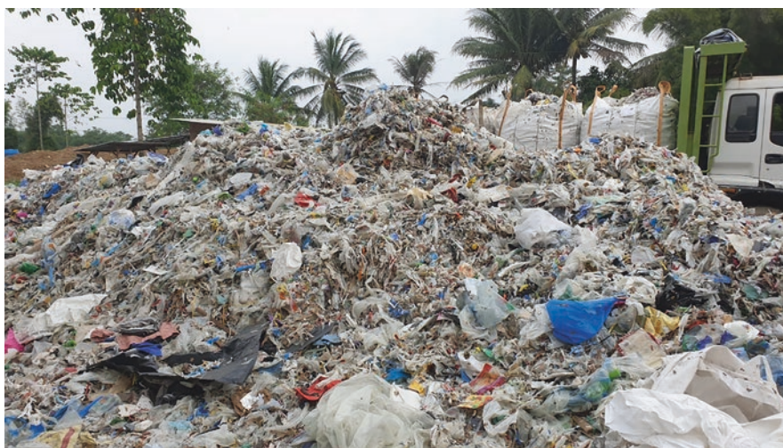
Fig. 8 Plastic waste contaminants from one paper mills in Karawang, Indonesia, to be transferred to lime burning plants near the factory. (Photo credit: Tio Septiono)
