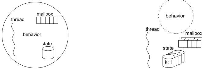
(a) Non-virtual actor: coupled mailbox, thread, behavior, and state. (b) Virtual actor: fully decoupled and externalized mailbox, thread, behavior, and state.
