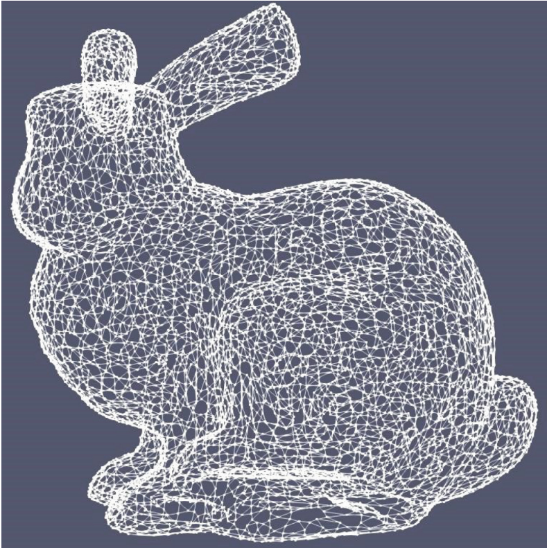
Fig. 2. An example of an unstructured surface mesh “Rabbit”.
