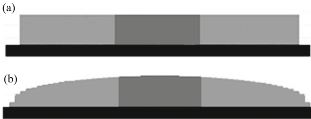
Fig. 2. Microsections of model splat morphologies (black color – substrate; dark gray shade – splat core; light gray shade – peripheral annular splat part): (a) – disk (cylindrical splat); (b) – smoothed splat, equivalent in volume to disk splat [6].
