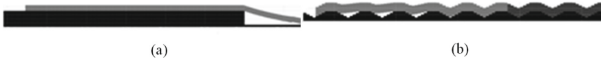
Fig. 3. Laying of the cylindrical splats (of gray shade) on a surface with a non-smoothed (variable) relief (black color): (a) – stepped relief; (b) – wave-shaped relief [6]. (Color figure online)
