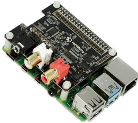
Fig. 2. Raspberry Pi 4B with HiFiBerry DAC + ADC Pro sound card attached on top.
