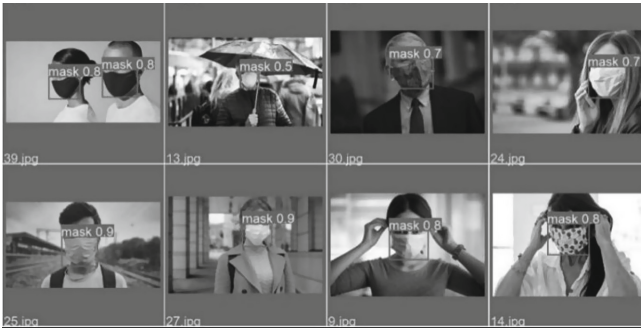
Fig. 9. Sample trained dataset with bounding boxes and mask prediction scores.
