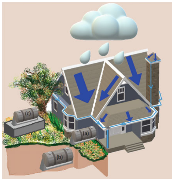
Fig. 3 General diagram of roof precipitation harvesting systems and possible storage locations. Source Created by Yasemin Kuslu
