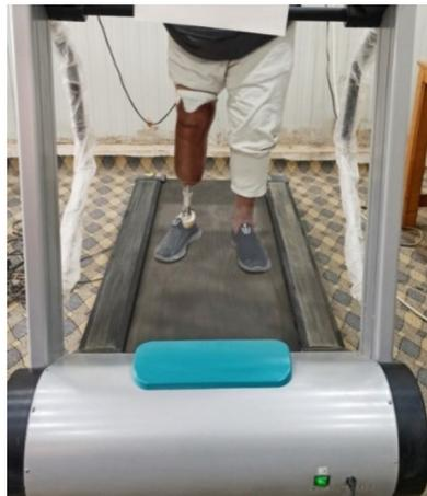
**Fig. 4.** In-Patient force plate walking test for the artificial limb using Treadmill.
