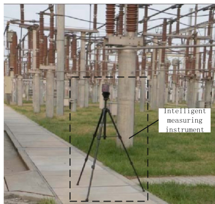
Fig. 8. Real scene layout of power frequency induction electric field intensity measurement points
