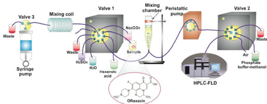
Fig. 10.6 The manifold for automated EA-SS-LPME system coupled with HPLC-FLD for the determination of ofloxacin in human urine samples. Reprinted from [84] with permission from Elsevier
